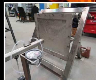
Bleed Air Leakage Test
