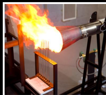
Kerosene Fuel Burner
